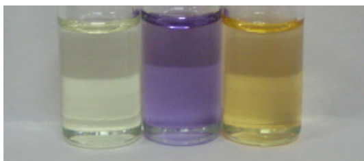
Fig. 3 Color changes of the receptor 1 ( 2 \times 10^{-5} M) with different acetate concentrations in DMSO. From left to right: (a) only 1 ; (b) 1.0 equiv. of \text{AcO}^- ; (c) excess equivalent of \text{AcO}^-
